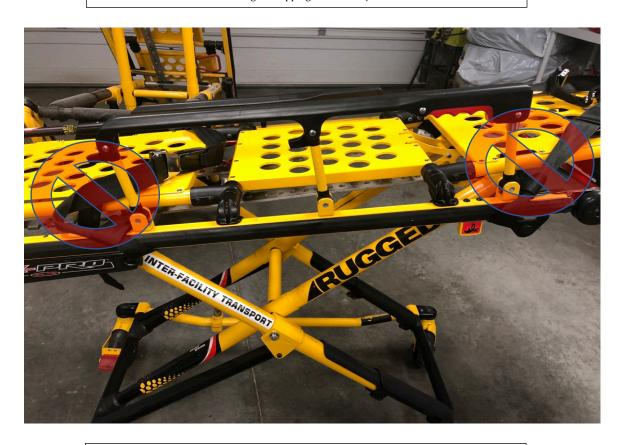
The illustration below should be common practice to install safety belts on each stretcher. By inserting the safety belts into the linear grooves on the adjustable frame, would allow you to utilize the foot/leg rest and backrest adjustments securely without compressing the abdomen and/or legs in the process.
