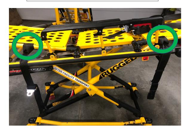
For the stretchers that currently feature a third, mid-section lap belt, the illustration below would be the proper position to install the safety belt. By installing the belts in this position would NOT affect the patient should she/he want their legs or head to be raised or lowered for comfort.
